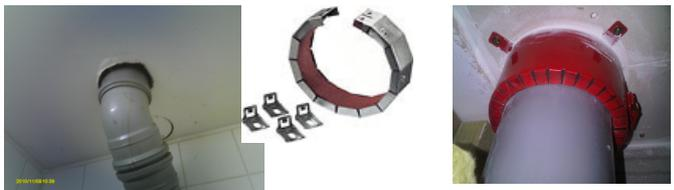
Intumescent collar for fitting round pipe through wall. The collar is lined with a fireproof material that expands in response to heat and blocks the hole by crushing the plastic pipe and expanding into the gap
